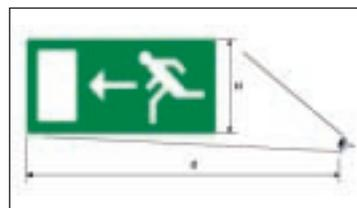
Figure 2 - Maximum viewing distance for Fire Safety signs
